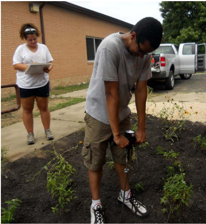
A hand-held penetrometer being used for precise measurements of soil compaction in a rain garden. The device is about three feet tall and has a dial on the top that reports soil strength in pounds per square inch. Photo credit: Rutgers Cooperative Extension Water Resources Program.
